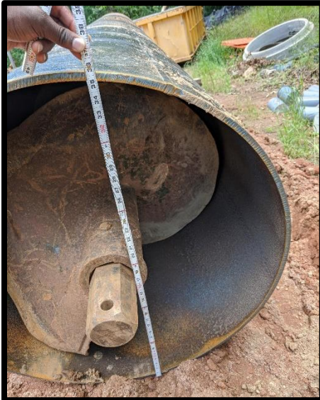
The image above illustrates the inside diameter of a steel casing pipe.
